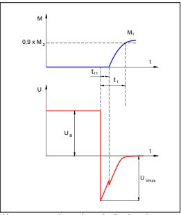
$U_B$  operating voltage (coil voltage)  $U_{Vmax}$  turn-off voltage
