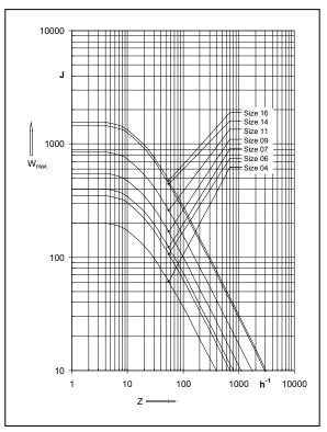
Fig. 38/1: Max. switching work W<sub>max</sub> per switching operation as a function of the number of switching operations per hour Z (values based on n=3000 rpm; applicable to dynamic brakes)
