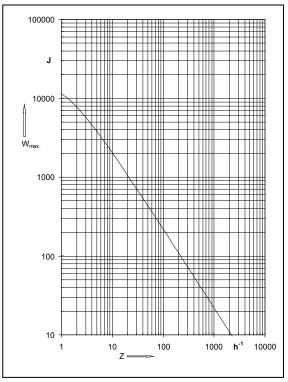
Fig. 24/1: Max. switching work  $W_{\text{max}}$  per switching operation as a function of the number of switching operations per hour Z (values based on n=1500 rpm)
