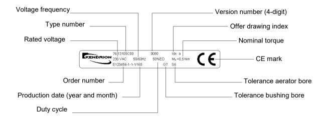
Note: The product number of the spring-applied single-disc brake consists of the type number followed by the version number, e.g. 76 13105C00-0080.
