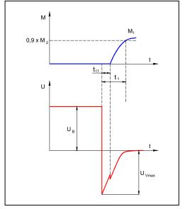
$\begin{array}{ll} U_B & \text{operating voltage (coil voltage)} \\ U_{Vmax} & \text{disconnection voltage} \end{array}$
